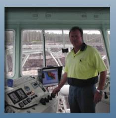
Trimble heading receivers provide precise navigation that is vessel-centric. Marine operators receive simple forward/back, port/starboard, and clockwise/anti-clockwise guidance, which allows them to position the vessel guickly and efficiently.
