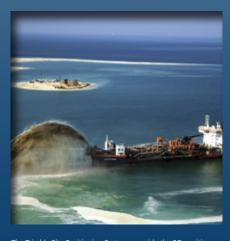
The Trimble Site Positioning Systems provide the 3D position of the dredge head and displays it with the channel design. Precise information gives marine operators "eyes under water", to see exactly where material should be dredged.
